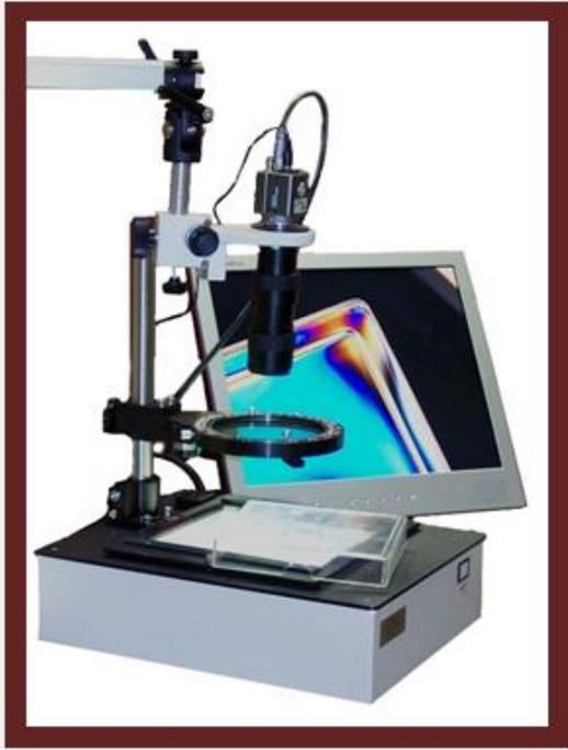
The PS-100-DIGIVIDEO Polarimeter system is the ideal solution for measuring **and digitally storing** residual stress or birefringence information from a wide variety of applications and industries. Its uses range from simple inspection and interpretation of photoelastic colors to precise quantitative measurements using analyzer rotation or compensation techniques.
