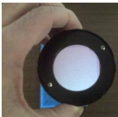
The **SWF-100** standard wavelength filter (left) assists in visualizing orders of magnitude of stress (fringes) in areas of high stress density. May be ordered as either a handheld accessory or attached to analyzer.
