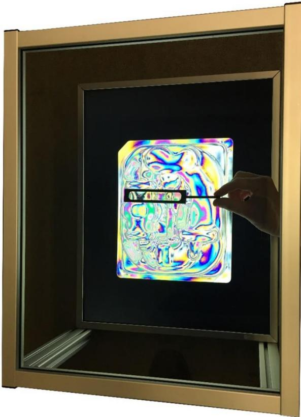
*Residual stresses are introduced by nearly every manufacturing process, including molding, extrusion, thermoforming, or joining with dissimilar materials. If not controlled, stresses can cause costly product failures due to surface cracking, warpage, delamination, and structural weakness.*
