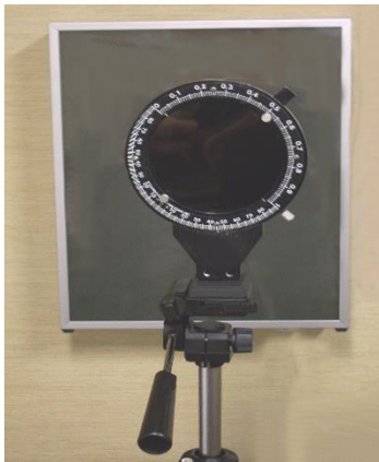
PS-100-LF , Horizontal Light Path Plane Polarization Only
